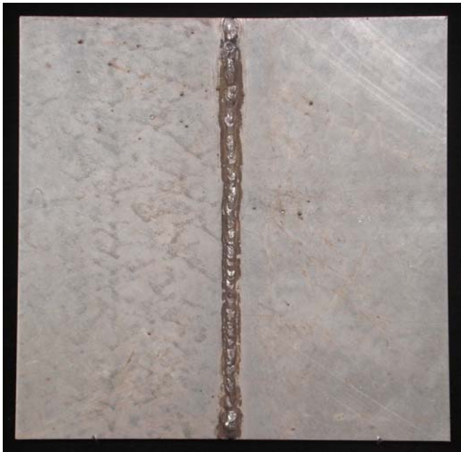
Figure 3 Showing a representative test piece after MIG welding.
