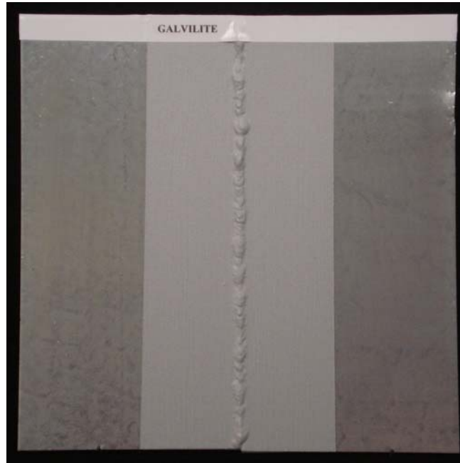
Figure 5 Showing test piece after application of Galvilite.
