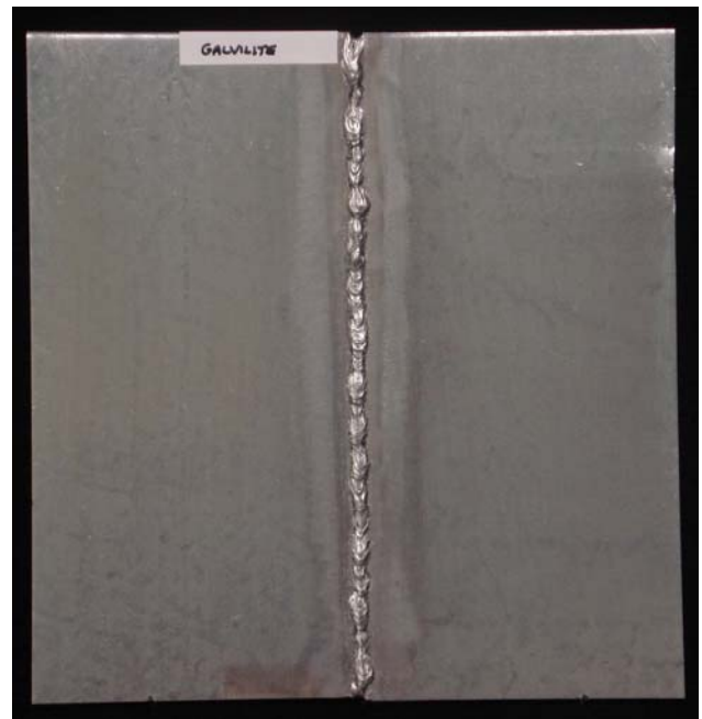
Figure 4 Showing Galvilite test piece after surface preparation.
