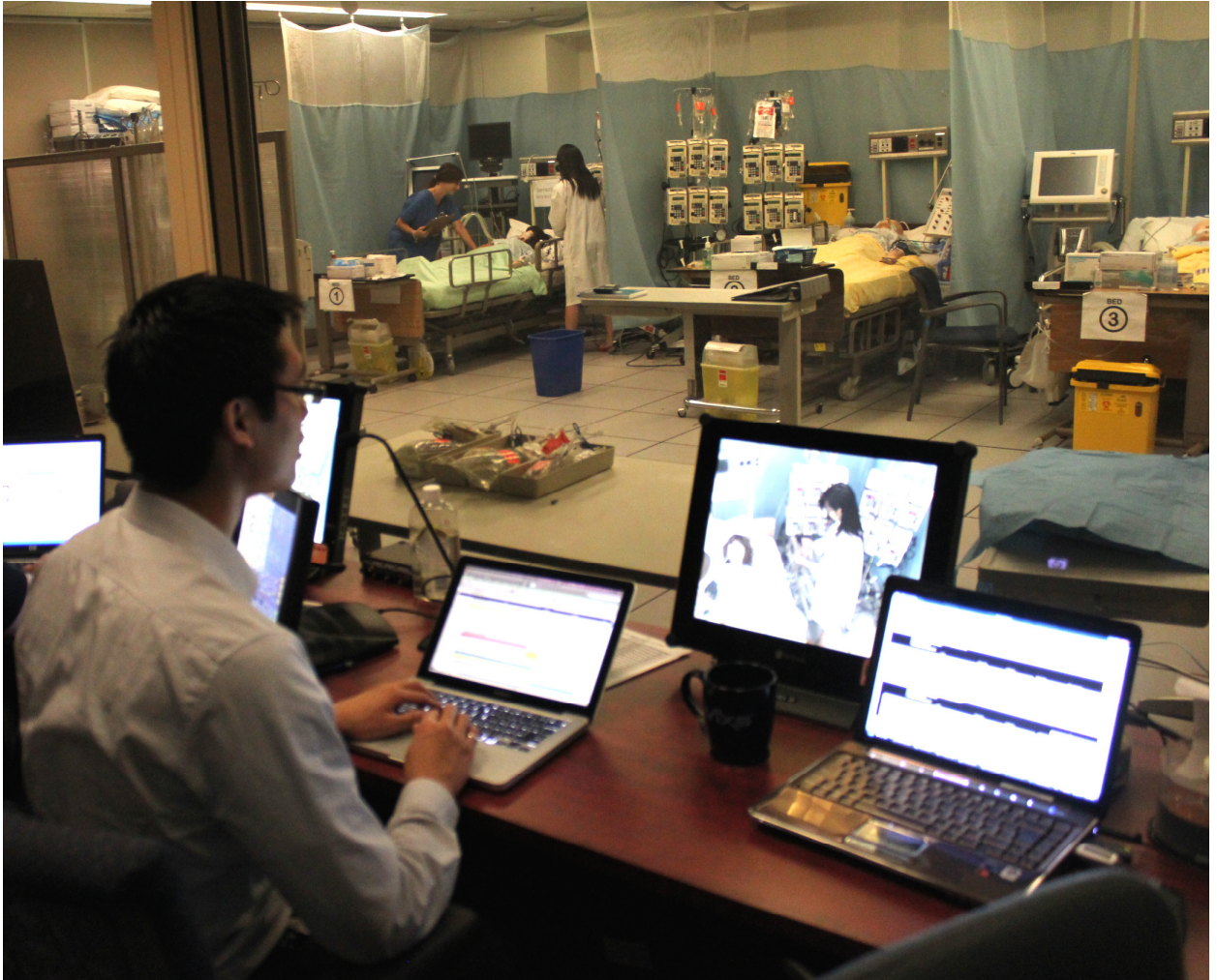
A Human Factors Engineer collects usability data on multiple intravenous infusion safety during a lab-based simulation with nurse from an intensive care unit.
