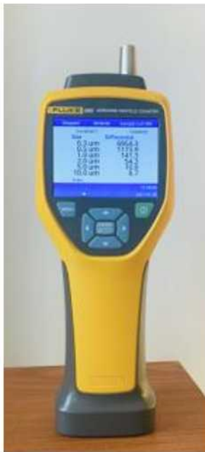
Figure 1. The particle counter, measuring the number of particles per liter of air of a given size indicated in the display. When aerosols are produced, these are visible as an increase in the different channels over the background (dust) particles. The average size of aerosols produced by human activity is around 5 \mu m [9], after evaporation of the water contained in saliva this gives rise to aerosols of about 1-2 \mu m. We thus use this size range also for the production of the artificial aerosols; the measurements presented below show the data for the 1 \mu m channel, however other channels give similar results and especially the same persistence time to within the experimental accuracy.
