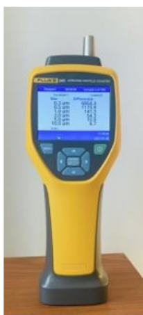
Figure 1: The particle counter, measuring the number of particles per liter of air of a given size indicated in the display. When aerosols are produced, these are visible as an increase in the different channels over the background (dust) particles. The average size of aerosols produced by human activity is around 5 \mu\text{m} , after evaporation of the water contained in saliva this gives rise to aerosols of about 1-2 \mu\text{m} . We thus use this size range also for the production of the artificial aerosols; the measurements presented below show the data for the 1 \mu\text{m} channel, however other channels give similar results and especially the same persistence time to within the experimental accuracy.
