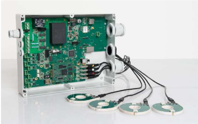
PMU-Device: Measuring U , I , \varphi every second
