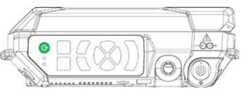
When used near an outlet, the EVO<sup>®</sup>/EVO<sup>®</sup> II system can be powered directly [with or without the internal Li-Ion battery pack installed] by the external power supply/ battery charger. It may also be used outdoors [unsheltered locations] as an internally powered system with a charged internal Li-Ion battery pack.
