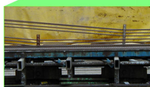
Hold down anchored to rail under bed
