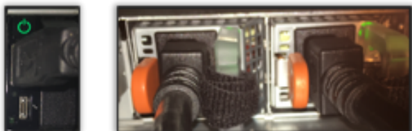
Redundant Power Supply
