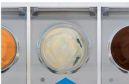
**Static Storage.** At the end of the batch freezing cycle, the Gelato is automatically stored inside the cylinder and ready to be served. There is no need to extract into another container and blast freeze it since there is no thermal shock. The ideal storage temperature for each flavor can be independently set and adjusted at any time.
