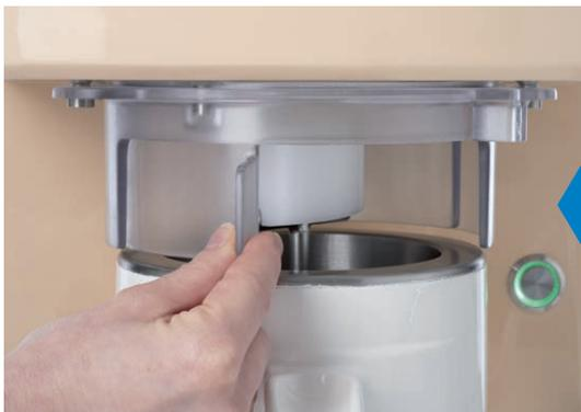
The beater stops immediately if the **protective lid** is removed during freezing.
