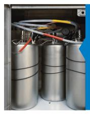
Pressurized system for dispensing syrups, the machine feeds three containers in the lower part for specific syrups with the desired flavor.
