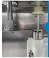
Automatic delivery closure. This machine is equipped with a portion control. The system delivers the correct portion required, regardless of the size of the cup.
