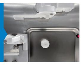
Protective casing of the actuator dedicated for automatic production. Prevents any interference from the operator.
