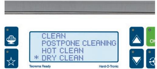
Once washing has been completed, all humidity can be eliminated from the cylinder with the **drying program**, essential before tempering chocolate.
