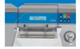
The sprayer is located on the front panel of the machine for easy cleaning of the cylinder and the chute, and to avoid having to cross over the door. The sprayer can also be locked to facilitate handling during use.
