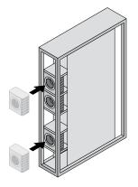
To achieve the max. cooling output of 30 kW, the customer/ service should install two additional fan modules.
