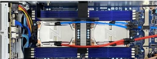
As a reminder, even with direct-to-chip cooling, not ALL of the heat generated in an individual chassis will be removed. There will still be the need to remove any remaining heat generated by the other subsystems (power supplies, other boards, etc.) in the chassis not supported by the DTC system.
