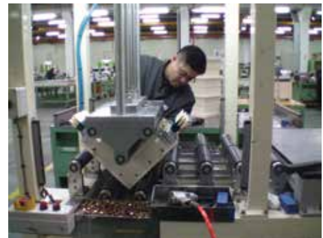
ASSEMBLY EQUIPMENT AUTOMATIVE (ONLY SCREW MANUALLY BY AIR HORSE)
