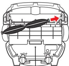
5 Press the Brush to the right and insert the left side of the Brush into the socket.
