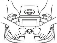
3 Gently lay the machine on its side so that the side with the dustbin is up
