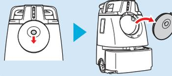
2 Check that the Dustbag is installed and the Dustbin pin is afloat
