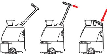
2 Hold the lift handles with one hand, and hold the steering handle down with another hand
