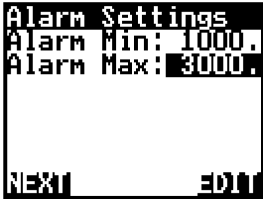
Wizard or manual alarm points. Example of a Shaft Alarm set at Min of 1000RPM & Max of 3000RPM
