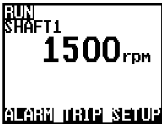
Example: 1UP monitoring 1 shaft
