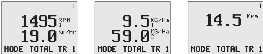
Figure 41: Example of main screen and secondary information screens as the MODE button is pressed when configured as an Airseeder monitor as described in this section
