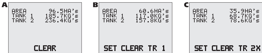
Figure 42: Example of the TOTAL (A), TRIP 1 (B) and TRIP 2 (C) (currently active trip, indicated by the X) screens for the Example Airseeder configuration
