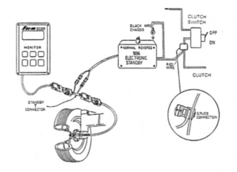
The 1036 ELECTRONIC STANDBY connects to any existing switch that is turned on or off when the machine is engaged (eg. clutch switch).
