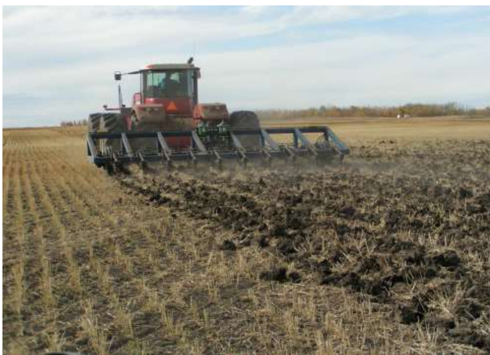
AP 70 Series Agrowplow Fitted with Hydraulic Recoil Shanks
