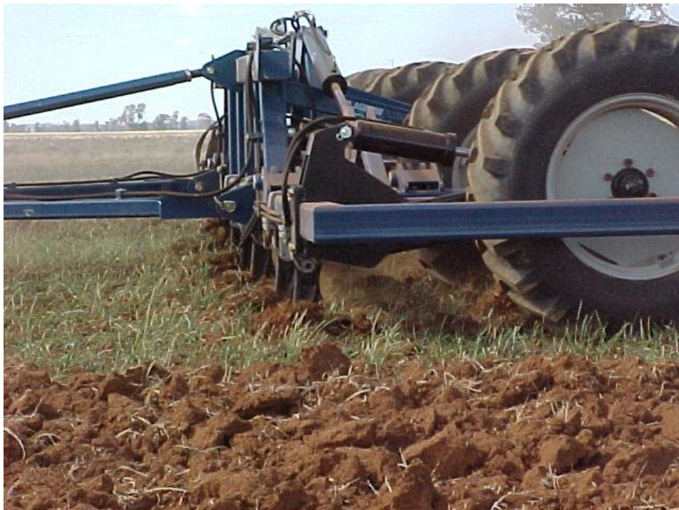
Figure 5.1: Correct soil moisture content is important to achieve shattering.
