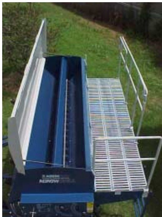
Figure 5.4: 3000 Series Agrowdrill seed and fertiliser hoppers
