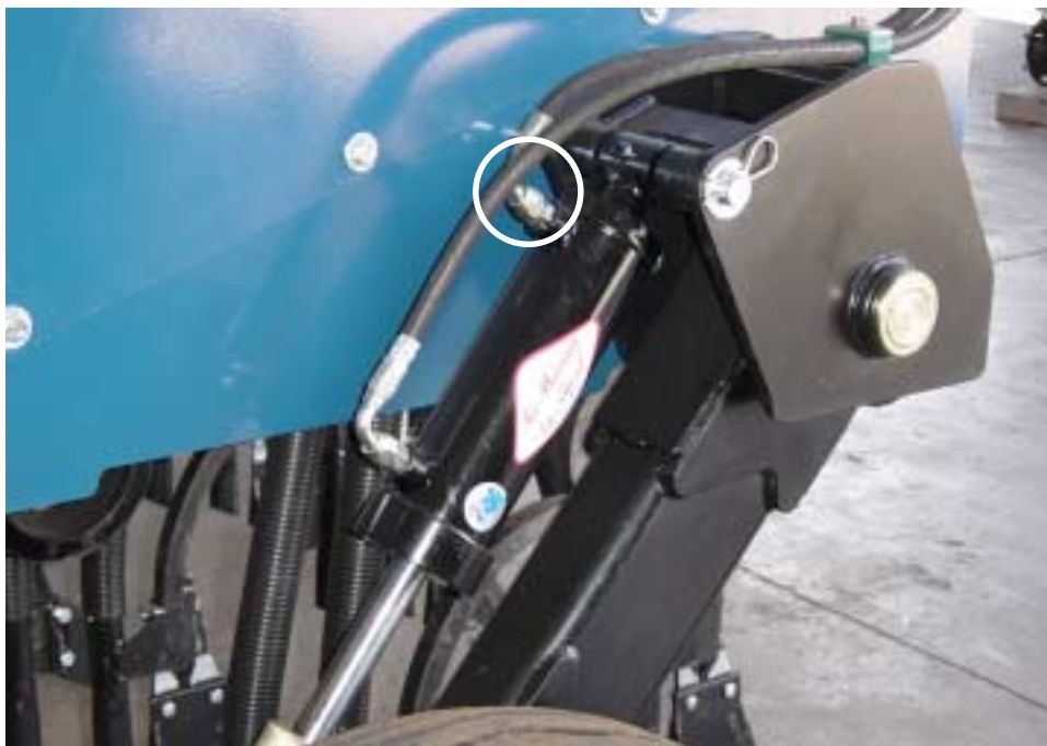
Figure 5.2: Right Hand Wheel Lift Cylinder
