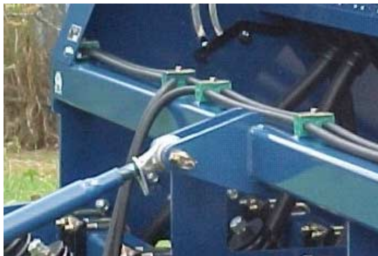
Figure 5.1: Levelling tube top connection
