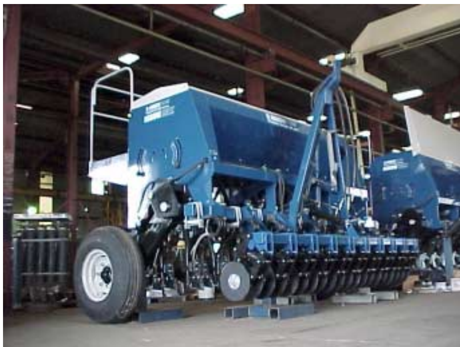
Figure 5.3: A coulter equipped 3000 Series Agrowdrill
