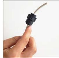
4. Insert the **Ethernet Cable Gland** provided in this package
