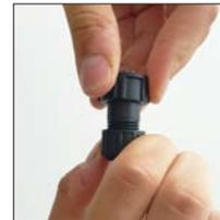
11. Insert the connector in the ethernet cable gland
