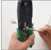
2. Use the crimping tool to cut one end of the ethernet cable
