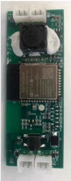
Figure 4 -PCB: LWS-TW6 Double Port Controller Board
