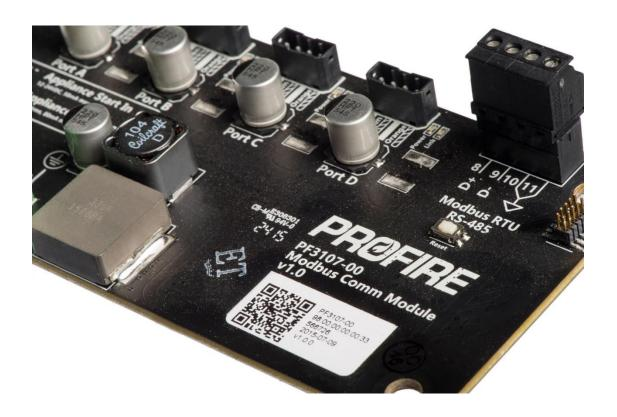
The PROFIRE PF3100 IO Modbus RS-485 card allows a PF3100 system to interact with other devices.
