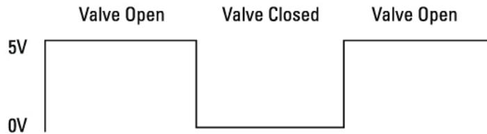
**Figure 19 - Level Based Valve Output**
