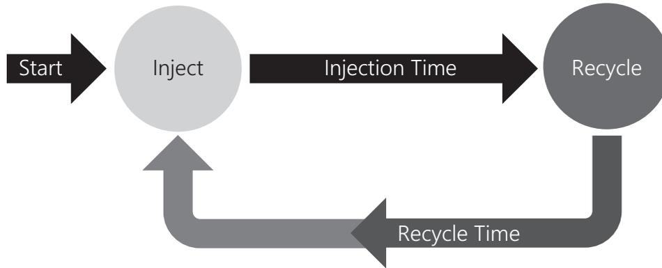
**Figure 10 – Single Pump Injection**
