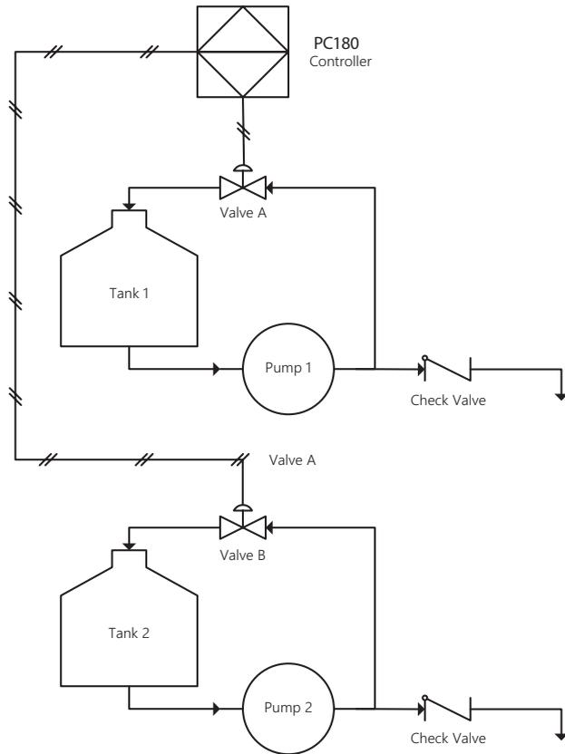
Figure 11 – Dual Pump Injection
