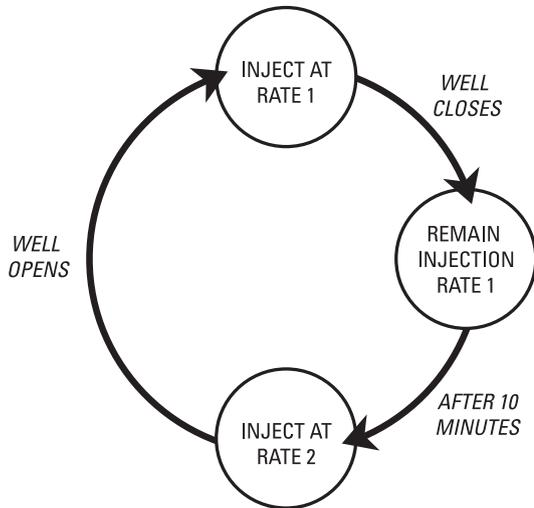
**Figure 17 - Artificial Lift Optimization**
