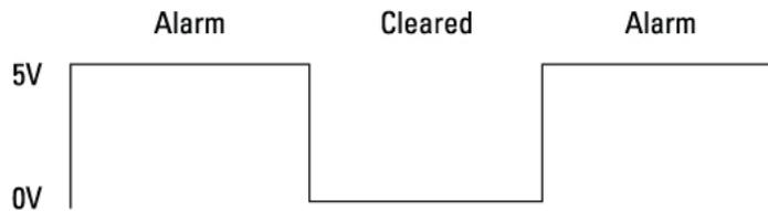
**Figure 20 - Level Based Alarm Output**
