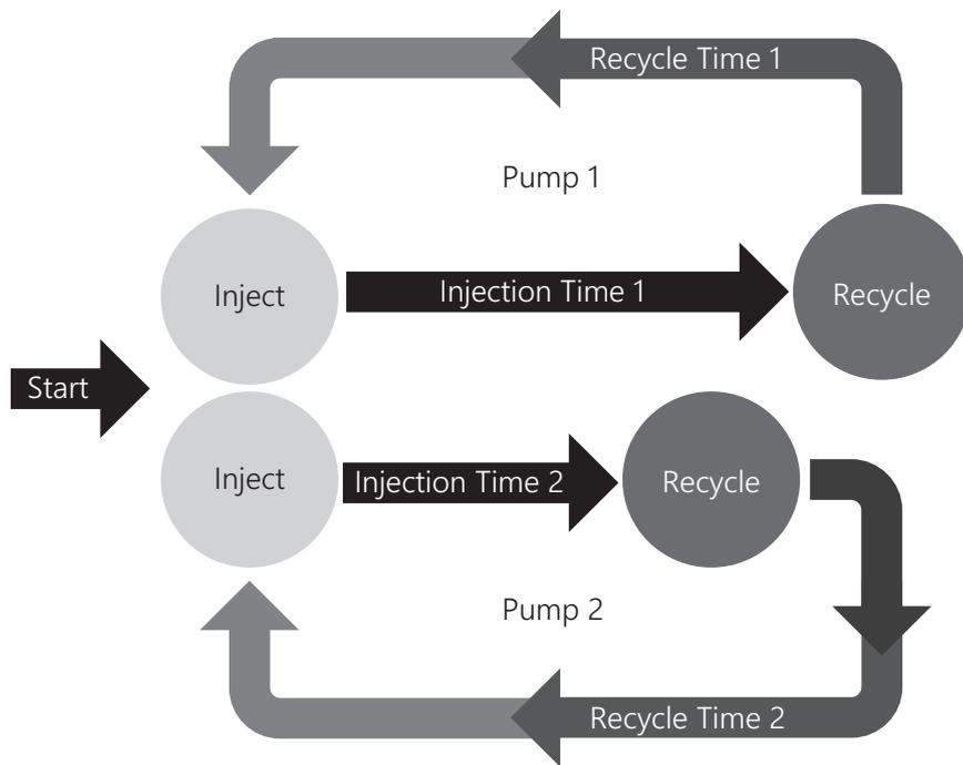
**Figure 12 – Dual Pump Controller States**
