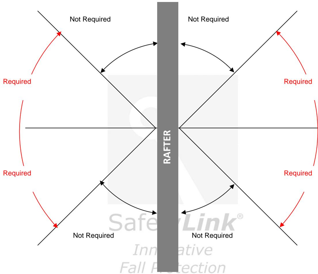
Install anchors only to Steel Frames strong enough to support the anchor point. Minimum Steel Frame size is 70mm by 35mm 0.75mm thick. Inspect the Steel Frame for damage. Ensure the structure is secured in accordance with Industry Building Codes.
