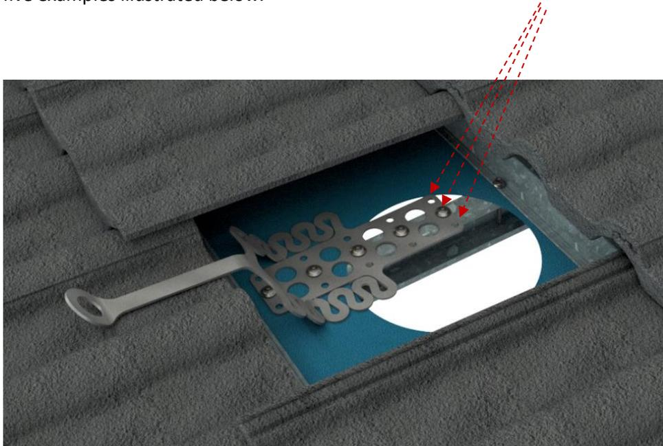
3. If the anchor point has a possibility of taking a fall in a direction 45 – 90 of the rafter additional lateral bracing may be required to support the rafter from side loads.
