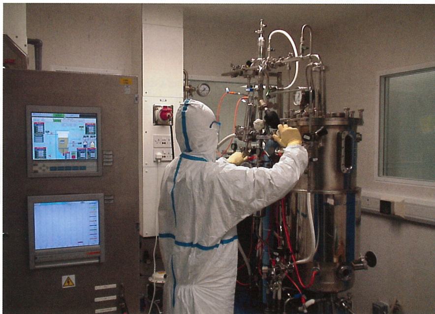
Upstream processing at Cobra Biologics... 50L Microbial fermentor
