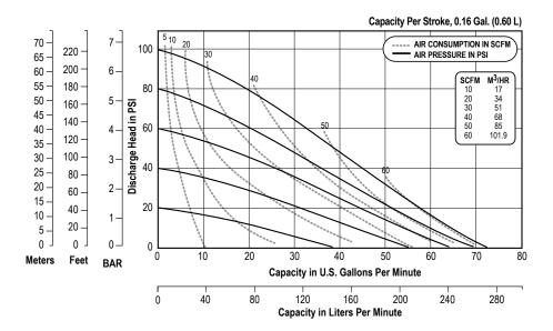
NOTE: Performance based on the following: PTFE fitted pump, flooded suction, water at ambient conditions. The use of other materials and varying hydraulic conditions may result in deviations in excess of 5%.
