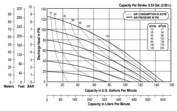
NOTE: Performance based on the following: elastomeric fitted pump, flooded suction, water at ambient conditions. The use of other materials and varying hydraulic conditions may result in deviations in excess of 5%.
