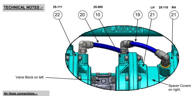
When looking from the air valve side of the pump, air hoses (items 19 & 20) are connected as shown. Inner chamber LH (22) connects to LH spacer chamber (21) and inner chamber RH (10) connects to RH spacer chamber (21).
