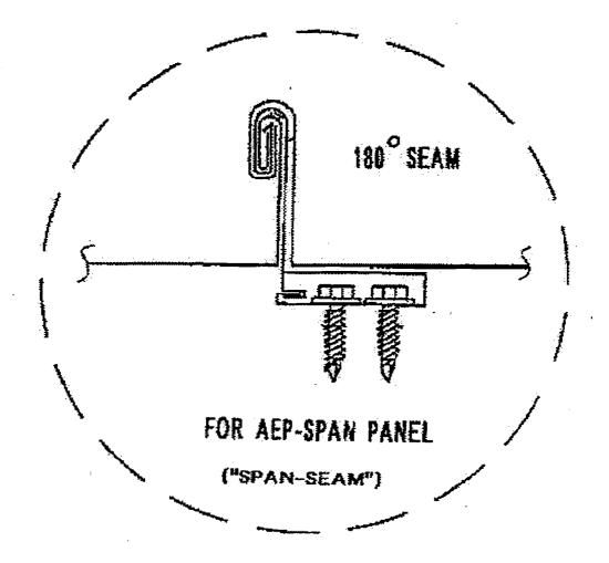
1. Metal Roof Deck Panels\* — No. 24 MSG min gauge coated steel, max width 16 in. Panels continuous over two or more spans. End lap to occur over purlins and to include End Lap Back-up Plate (Item 2B or 2C.) Ends of panels overlapped 6 in. Side laps to be tightened and crimped with a special motorized crimping machine at a minimum 45 degree angle with crimping process to include tabs of Panel Clips (Item 2). A bead of sealing compound may be used at panel end and side laps.
