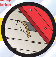
Sheathing and siding decay
