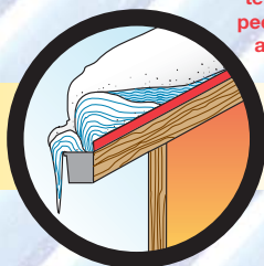
Improper attic ventilation causes snow melt under snow. When temperatures drop, melted snow freezes and backs up into roof seams
