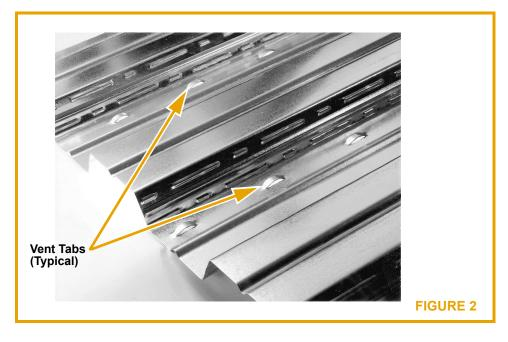
Vent tabs projecting upwards are staggered in interior low flutes at approximately 6 in. on center:
