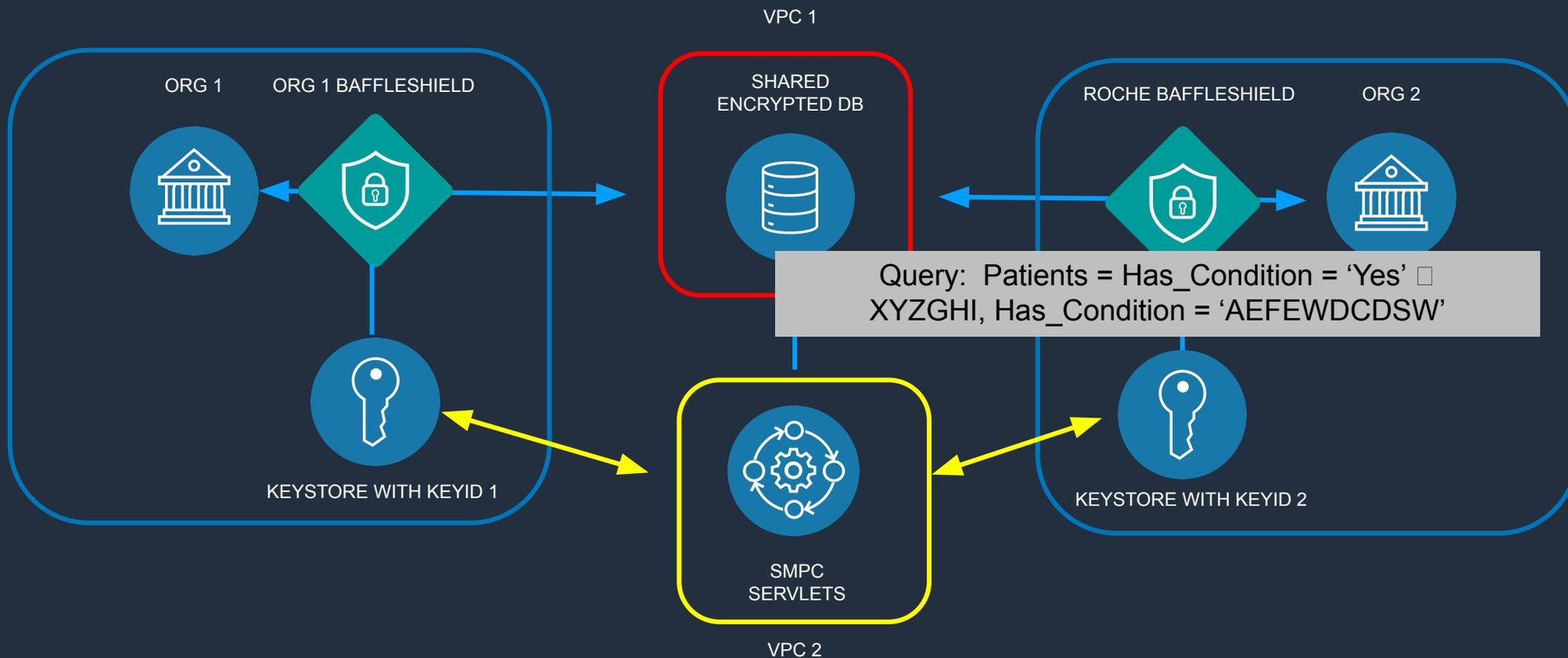
**4** SMPC performs a comparison operation on using different keys without ever accessing the encrypted data values. The results are returned without decrypting the data.
