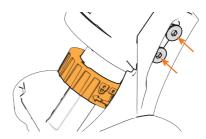
6 To adjust needle position, loosen the two screws under the injector (with a 2.5mm hex key), move accordingly and tighten to secure.
