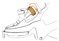
1 Detach fluid junction and needle from injector by rotating the orange lock nut and slide fluid junction forward to remove.
