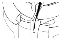
5 Check the position of the needle. When injector is fully retracted, the tip of the needle should be around 2mm inside the front pin.
