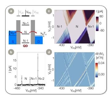
**Figure 4.** Coulomb blockade measurements. a) Schematic overview of the Coulomb blockade thermometry measurement. b) Plunger gate voltage trace at a 100  $\mu$ V source voltage, showing peaks in current where the single electron tunneling occurs. c) Current measured through the quantum dot as a function of the voltages applied to the plunger gate and source contacts. b) Differential conductance map measured simultaneously with c).
