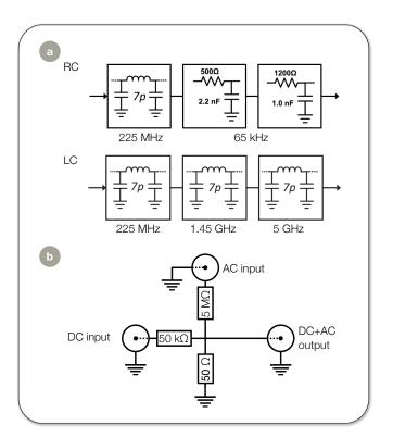
Figure 3. Electronics schematics. a) Schematic overview of the QFilter RC and LC filter banks. b) Schematic of the voltage divider used to apply DC and AC voltages to the source electrode.
