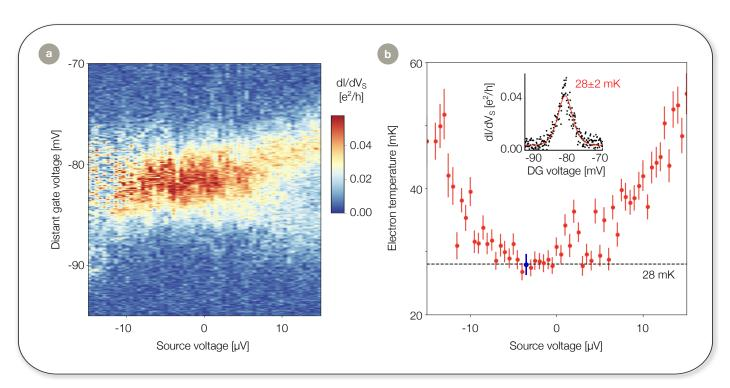
Figure 6. Electron thermometry measurement with further optimized parameters. a) High resolution scan of the Coulomb peak near zero bias, using a distant plunger gate and a voltage divider for the source voltage to increase the resolution. b) Measured electron temperature by fitting the Coulomb peaks with eq. 3 (see inset for the fit resulting in the blue datapoint). A black dashed line shows the measured electron temperature of 28 mK.
