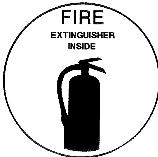
Figure 2-2: Portable Fire Extinguisher Location Label
