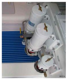
The fuel once flown through the separator pre-filters is still dirty, for this reason the engine is equipped with water separators, able to hold the remaining particles of dirt.
