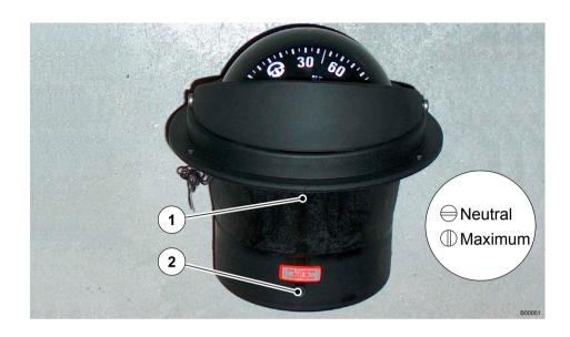
You compass is fitted with a set of compensation, or adjustment, screws to minimize these errors. It is seldom possible to compensate for all compass deviation errors, since this type of error varies as the heading of your vessel varies. However, the error should remain the same for any given heading, as long as no changes are made to instruments and electronic fixtures near the instrument panel.
