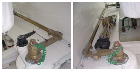
Cylinder, coupling rod and tiller angle indicator
