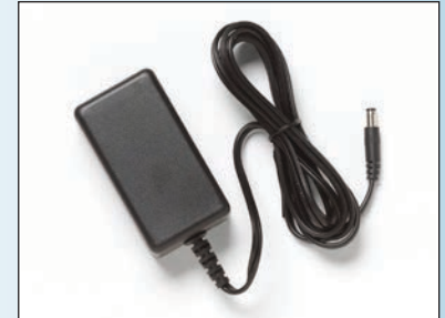
Part Number: 2647372 Description: BE-UNVSL-IEC320C14, BATTERY ELIMINATOR 90-264VAC/9VDC 1.7A CTR NEG
