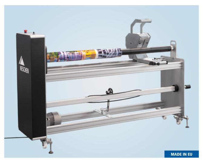
The Neschen Rollcutter 1650 has compact dimensions and thus it is perfect for even small workshops. Through its large 360 degree rotatable and wide rolls it can be easily (re-)placed.
