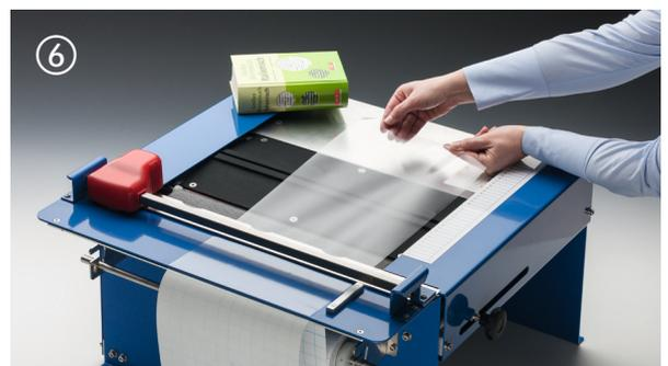
Pull the film off the roll to the measured coloured spot.
