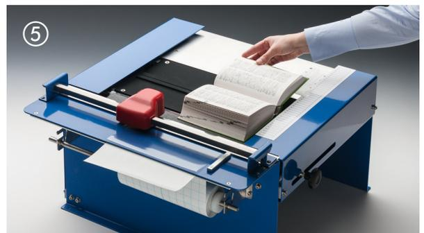
Please ensure that there is an overlap here, too, of 2 cm for the book cover. The distance between the edge and the head of the cutter should be about 2 cm. Open the book roughly at the middle and check the printed scale to see how much of the filmolux film you will need to pull off the roll.
