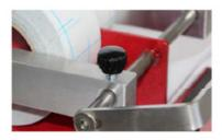
1. Loosen the knurled screw and slide the tape holder outwards.
