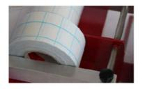
4. Secure the roll with the tape holder and tighten the screw. The tape can be cut off with a light diagonal, downward motion onto the cutting blade.
