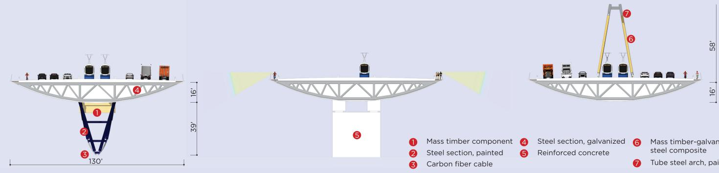
In our design approach, mass timber-steel composite hangers would create a unique aesthetic and texture on the bridge, and there is an idea that mass timber-steel composites can reduce the stress range in the hangers and potentially improve their fatigue performance.
