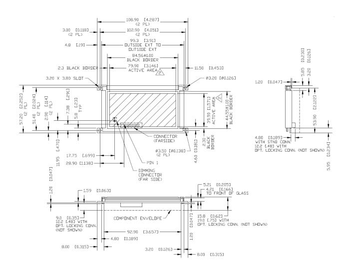
Dimensions in are millimeters; inches in brackets. Tolerances unless specified
