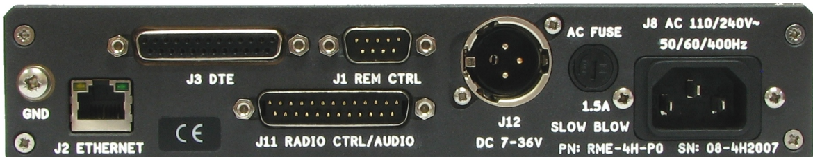
Fig2: Rear panel of the RM4 Unit
