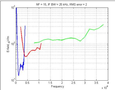
The graph illustrates the direction finding sensitivity of a typical system. The sensitivity is for an IF bandwidth of 25 kHz and without averaging. The graph depicts the minimum signal required to obtain a bearing fluctuation of less than 2° and a probability of wild bearing less than 0.1%.
