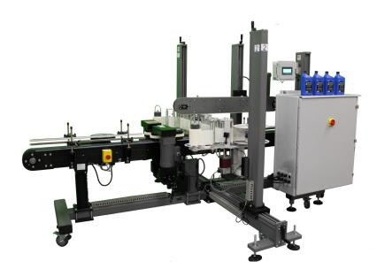
The 622W/T is a heavy-duty, affordable front-back labeling system. The compact size, durability, and low cost make the system ideal for small, medium or long-run jobs. Large volume, high-speed packing applications are handled with ease.
